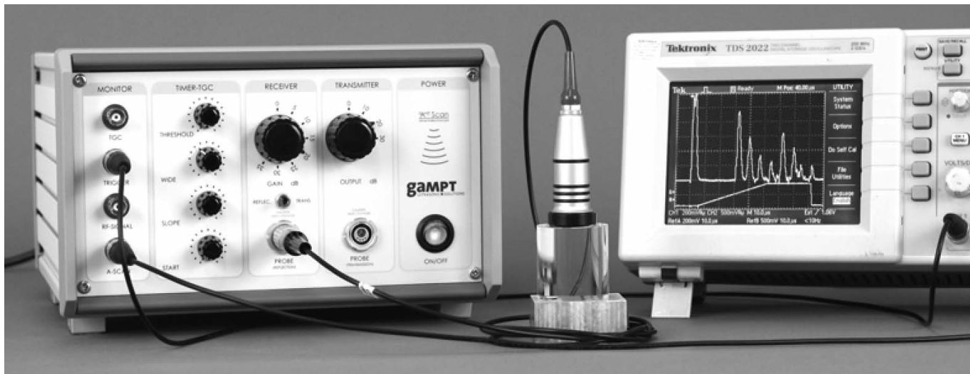
Fig. 6: The echoscope set-up
