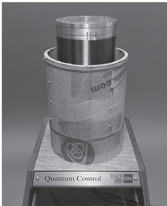
Fig. 2: A 'jury rig' of a dB_z/dz gradient coil, wound onto a cardboard tube, and put into place around the solenoid of a Quantum-Control apparatus.
