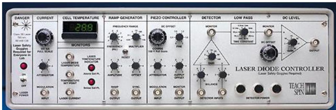
The ramp generator creates the changing voltage which powers the Piezo controller to vary the angle of the grating and thus 'sweep' the frequency of the laser. When the laser light reaches a 'resonant' frequency, photons are absorbed by the rubidium atoms decreasing the brightness of the transmitted light. The detector panel provides power for the detectors and offers extra signal manipulation.
