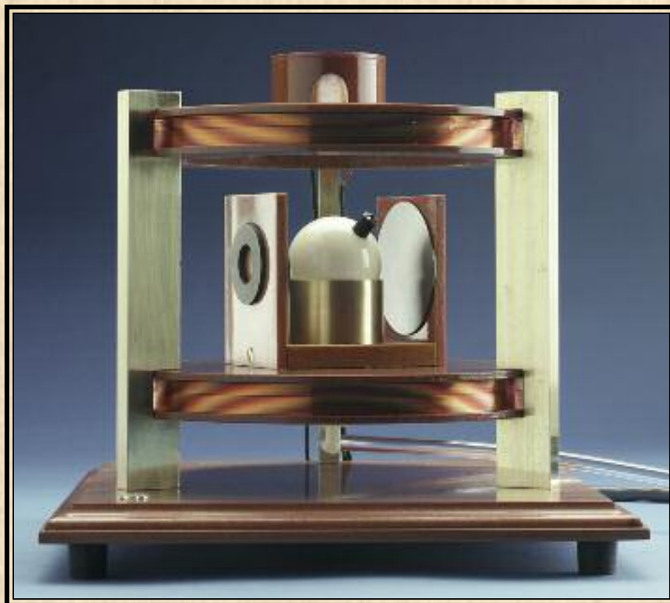
Figure 8 - Magnetic Torque with Rotating Field Attachment
