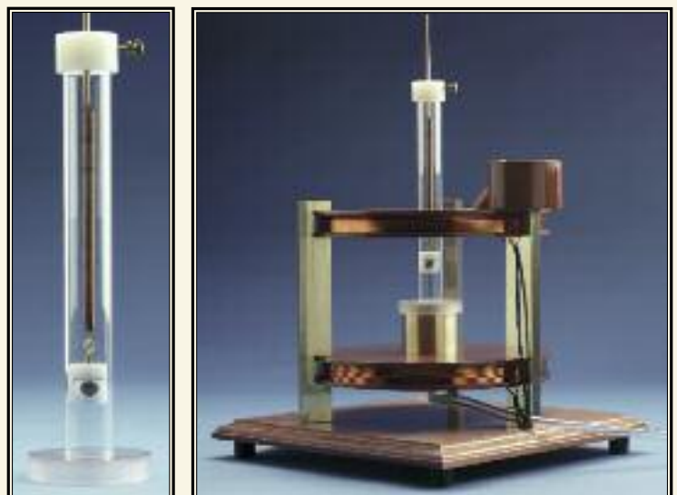
Figure 6 - Magnetic Force Apparatus with Detail of Gimbal and Calibrated Spring
